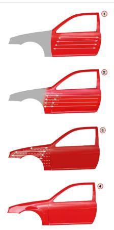
Begin by applying 1 - 2 closed coats of Permahyd Blend-in Additive 1050 / 1051\* to the blending area. Ensure that the blending area is large enough. Do not allow Permahyd Blend-in Additive 1050 / 1051 to flash.\*\*
