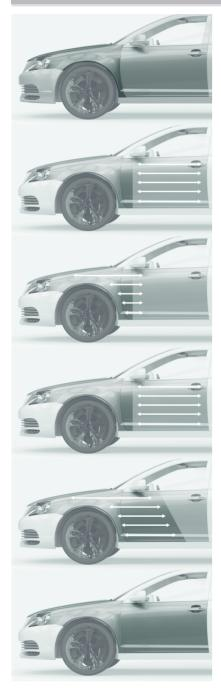
Adjacent panel: sand panel with suitable abrasive e.g. Trizact - P1000 New part / repair: sand surfacer (minimum P500)
